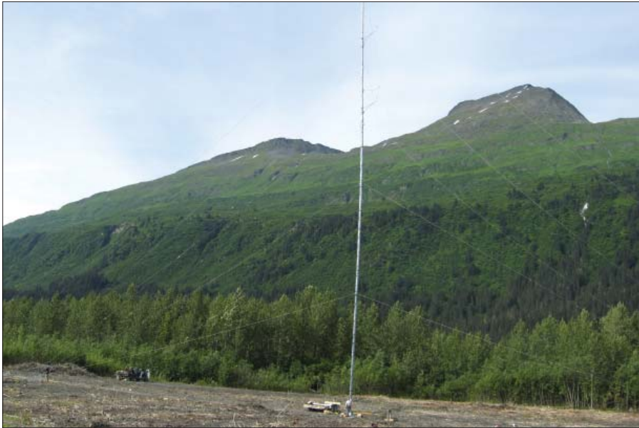
The CVEA MET tower that was located at 10 Mile in Valdez; data collected at this site determined the site was not good for a commercial wind generation project.
