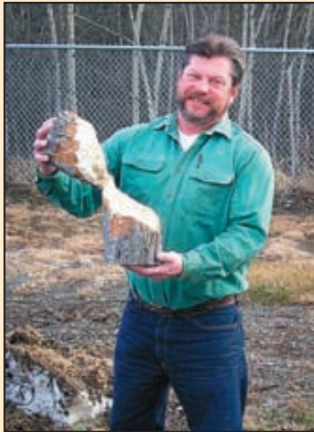
Above, Glennallen Line Foreman Mike Leeper shows the cause of a 2006 outage near Squirrel Creek. The beaver was not hurt in the incident. Opposite page, Terry Delay keeps a watchful eye on the power grid using the SCADA system.
